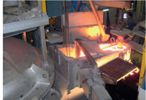
Pouring spout with float system and quickly replaceable stopper
