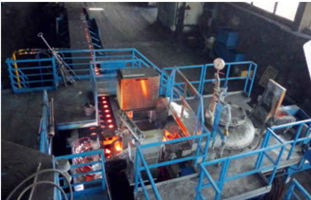
RGD 4/200 on a Disamatik moulding line
